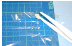
Substrate: Mylar (thickness 1.8 µm, greased with APIEZON L)
